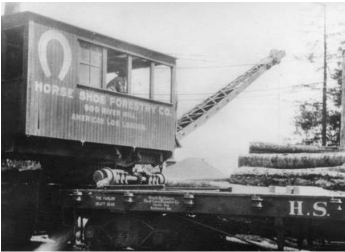
Figure 22. Log loader from the Horse Shoe Forestry Company's Bog River Mill mounted on a railroad flat bed. Courtesy of the Piercefield Museum.
