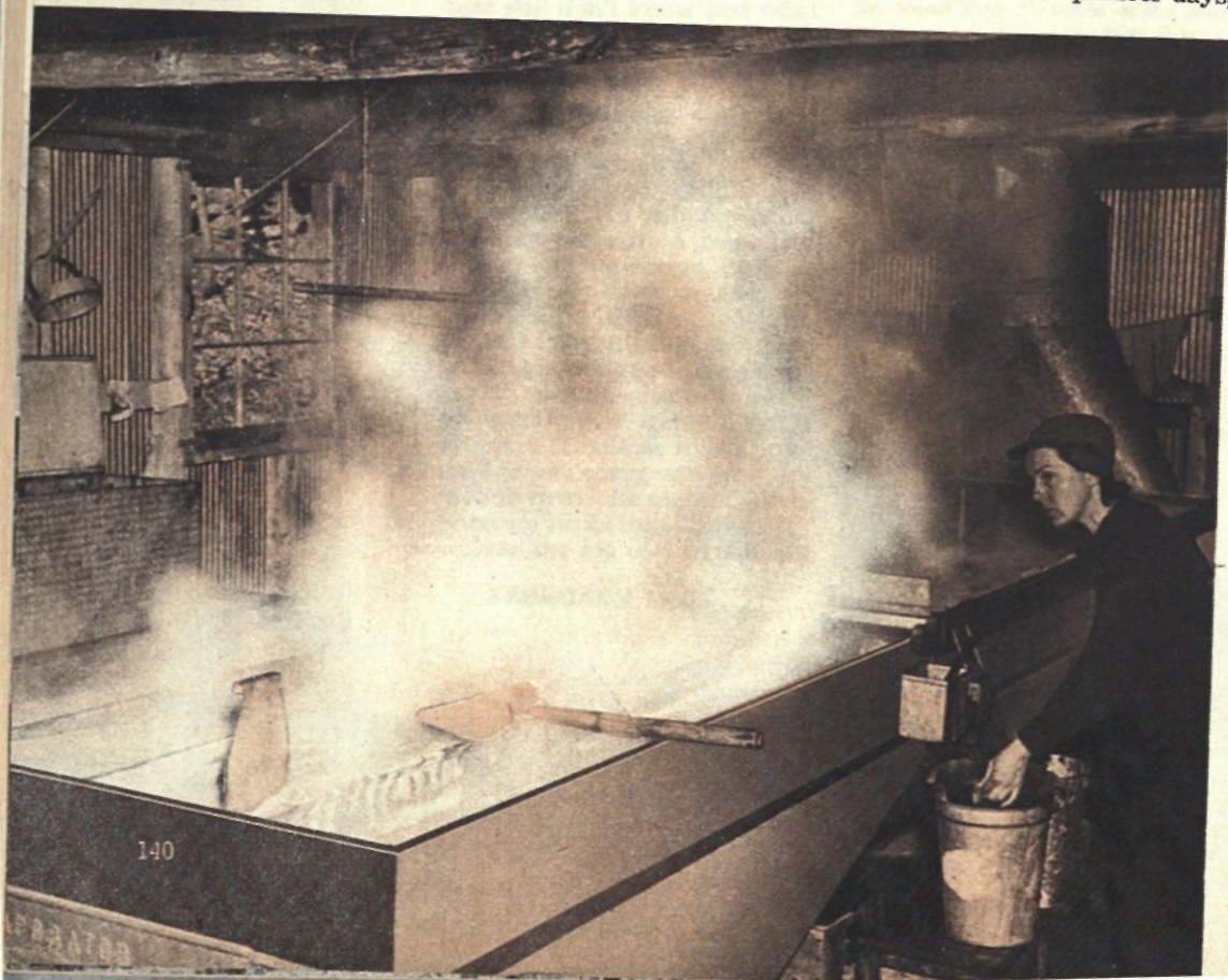
The old, and still reliable, way to tell when syrup has boiled enough is to see if it "sheets" when drained from this scoop. Below, Mrs. Helen Nearing helps out by running the evaporator
