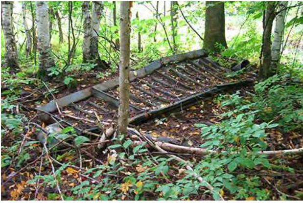
FIGURE 2.13. An abandoned early continuous flow flat-pan evaporator with partitions.
