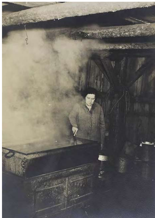
FIGURE 2.12. Katherine Skinner boils on a continuous flow evaporator on a metal frame wood-fired arch in Westmore, Vermont, in the 1940s. (GAUTHIER)
