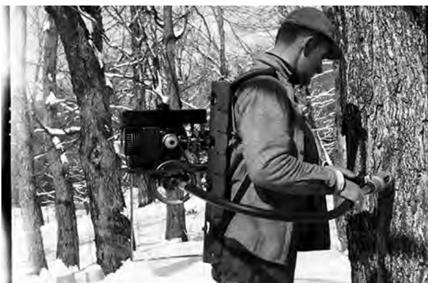
FIGURE 2.4. Gasoline powered tapper. (UVM LIBRARY SPECIAL COLLECTIONS)
