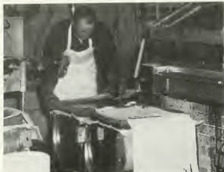
Figure 95.—A simple type of flat filter. A basket of hardware cloth is supported above the two tanks for holding the felt and above this is the support for the prefilter. The prefilter is moved across the tray as new filtering surface is needed.
