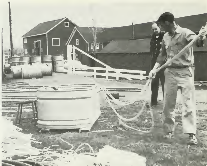
Figure 59.—The wash solution drains back into the tank as the tubing is slowly withdrawn.
