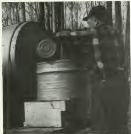
Figure 36.—Sap is easily poured from buckets into a low sump tank, from which it is pumped into the large tank.
