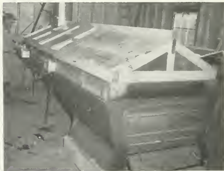
Figure 74.—The tight-cover steam-venting system with steam stack provides a simple, highly efficient means for removing steam. This results in a steam- and draft-free evaporator house.
