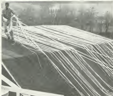
Figure 60.—The tubes are laid out on an incline or over a roof to drain. Here, 12 miles of tubing is being dried.
