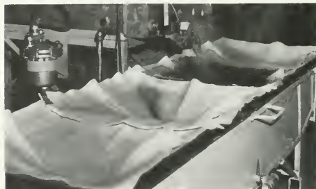
Figure 96.—A more elaborate type of installation in which three felt filter units are installed over a common tank. The units are mounted on rollers so that they can be replaced by a fresh unit when necessary. The tank is provided with a drawoff valve.
