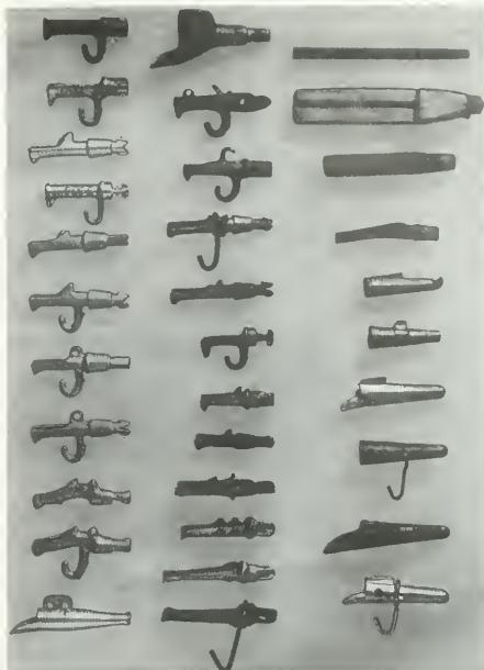
Figure 24.—Wood and metal sap spouts.
