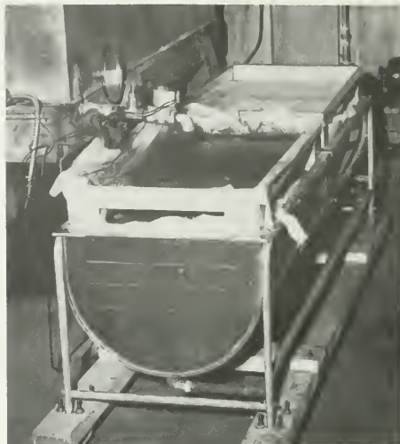
Figure 82.—The automatic drawoff is especially well suited for removing sirup from the evaporator. When a finishing pan is used, the evaporator functions as a semifinishing pan.
