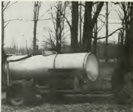
PN-4731 Figure 35.—For large operations or for collection from roadside trees extending along several miles of roads, the large tank trailer is desirable.
