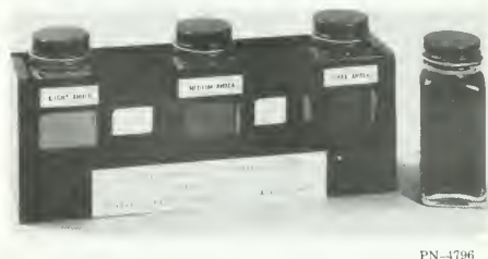
Figure 100.—Color-grading kit. The kit consists of the official USDA permanent glass color standard mounted in a comparator. The three clear blanks are in position in the comparator. For viewing, the sirup sample in the bottle to the right of the comparator is mounted in one of the two openings in the comparator.
