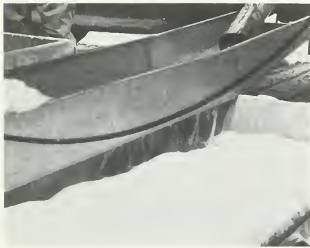
Figure 133.—Several layers of muslin or presscloth can be used to filter sap.
