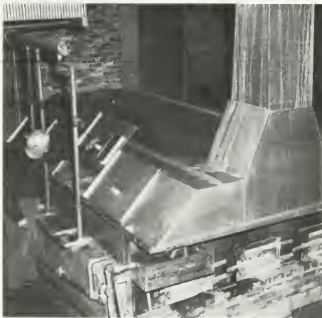
Figure 85.—A converted evaporator that uses high-pressure steam coils with steam generated by two 100-h.p. boilers.
