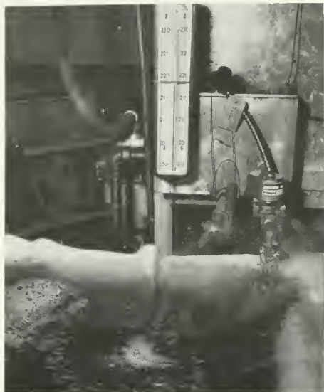
Figure 92.—The liquid-stem industrial thermometer has an open scale that permits calibration marks for each \frac{1}{4} ° F, and the temperature of the boiling sirup can be measured precisely. The thermometer is mounted outside the pan so it is not obscured by steam. It is especially suited when the pan is covered with a tight steam hood.
