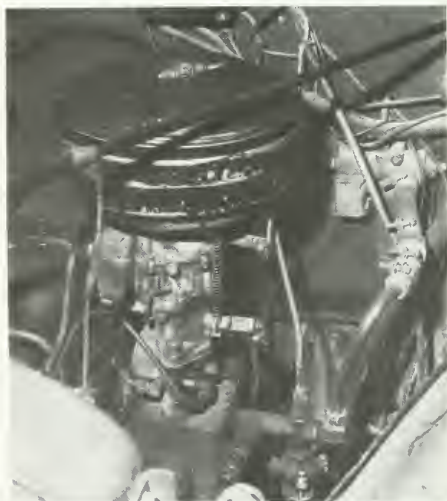
Figure 39.—The vacuum is obtained from the manifold of the truck engine.
