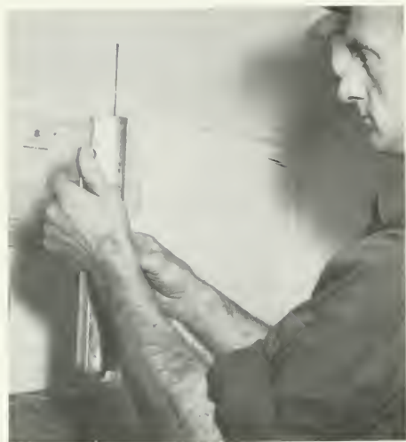
Figure 99.—A hydrometer is a simple, inexpensive instrument for precisely measuring the density (° Brix) of the sirup. The hydrometer should be read at eye level. The temperature of the sirup must be measured and a temperature correction made.
