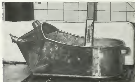
Figure 114.—A special candy-cooking kettle has one end shaped like a funnel and is provided with a spout and shutoff. After the cooked sirup has cooled but while it is still fluid, the kettle is mounted in an upended position and the sirup is run out through the shutoff. (Cookeer designed by Lloyd H. Sipple, Bainbridge, N.Y.)
