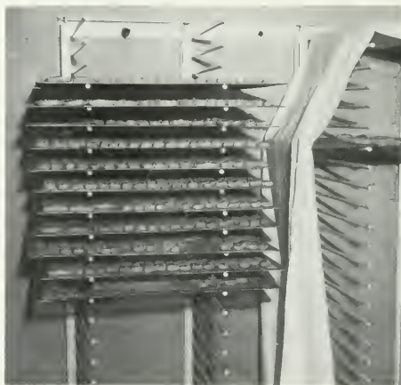
Figure 119.—After the candies have been removed from the crystallizing sirup and wiped, they are put on wire screen trays and placed in racks for air drying before packaging.
