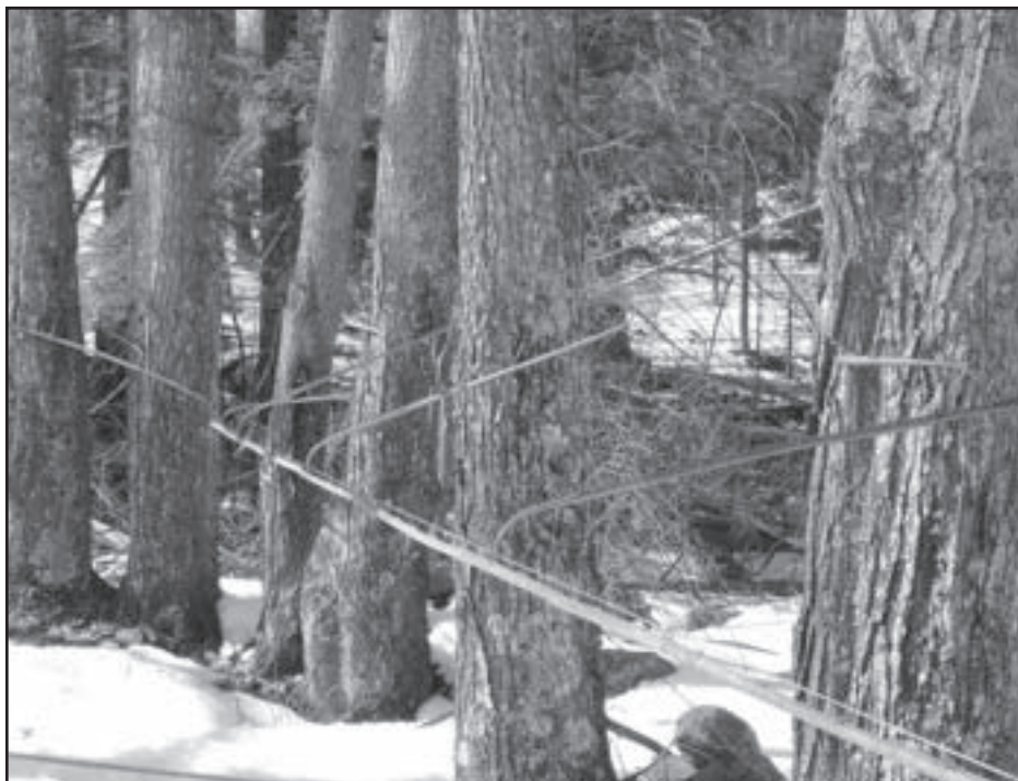
The Gooseneck metal sap pipeline in use during the 2005 sugaring season in the Lent Family sugarbush, Mayfield, New York. Copyright Matthew M. Thomas
